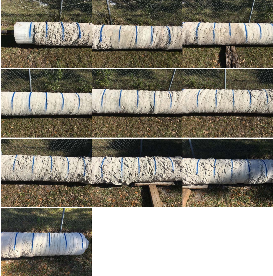
Figure 2.24 Extracted pile shape from top to bottom (left to right and down).
