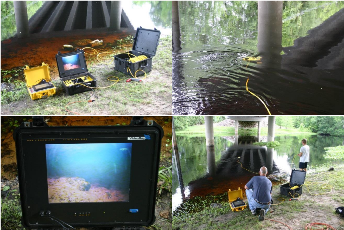
Figure 4.45 Remote operated vehicle system used to capture underwater images without divers.
