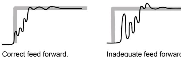
So look at feed forward as a form of a “predictor” of where the actuator should be going. The signal gives the servovalve an early indicator to tell it that it needs to open faster than would be expected from the existing error signal.
