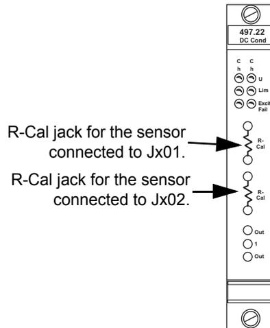
You also need to know which of the two DC conditioners on the module is used by your extensometer.
