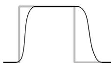
The shaded square wave represents the test command. The solid waveform shows an idealized feedback signal.
