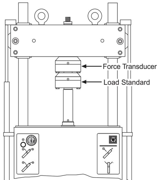
7. If you are using Gain/Delta K or Gain/Linearization for calibration, set initial conditioner calibration values on the Calibration submenu. A typical complement of ranges could be: 100%, 50%, 20%, and 10% of full scale. You can create ranges for any percentage of full scale. This creates a sensor calibration file and sets up any ranges you may want.
