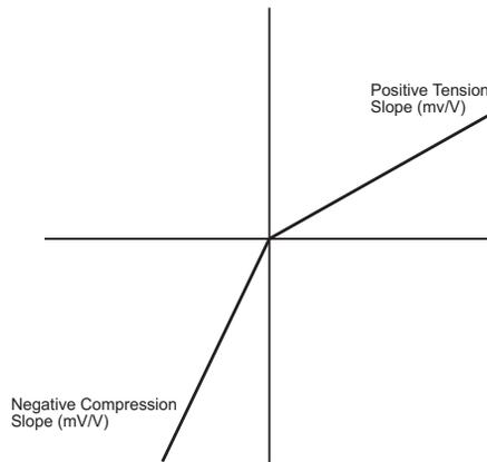
In this calibration process, system software calculates conditioner Delta K Gain and Gain values from previously measured mV/V values under both tension and compression.
