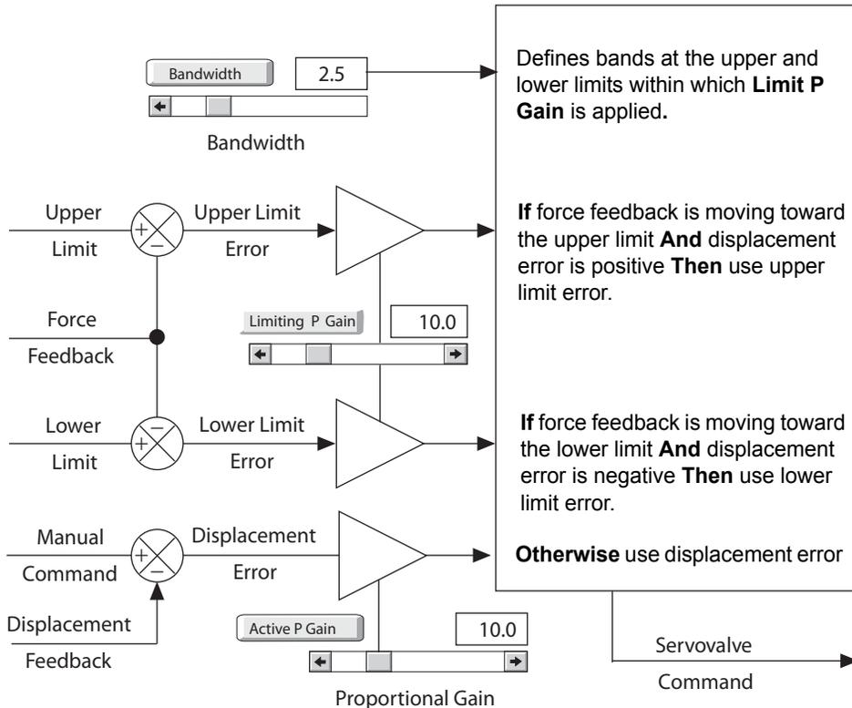
The CLC control mode uses one of three error signals. The **Limiting P Gain** adjustment acts as a conversion factor to scale the limit feedback to similar units as the active P feedback. The **Limiting P Gain** is turned on within the upper and lower limit bands defined by the **Bandwidth** control.
