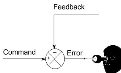
Integral (Reset) gain looks at the error side of the summing junction. It is the integral of the error, indicating the size of the error over time.
