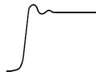
The same high gain signal after derivative gain has been applied. The derivative gain tends to damp out the ringing.
