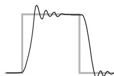
This waveform shows an unstable (high gain) feedback signal.
