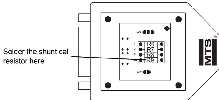
8. *FlexTest SE/LE, FlexTest GT, TestStar IIm Controllers only*: If you do not have transducer ID modules on your sensor cables, install the shunt calibration resistor as follows:
