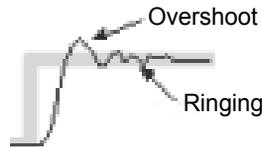
The middle waveform is a optimum waveform. In some cases the optimum waveform will have no overshoot or ringing, and the waveform will look more like a square waveform with rounded corners.
