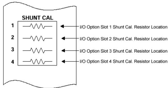
9. *FlexTest IIm/CTC Controllers only*: Install the shunt calibration resistor into the **R-Cal** jacks in the appropriate DC conditioner.
