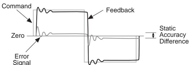
The square wave shape of the error signal represents the phase lag of the feedback signal.
