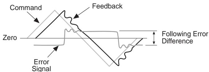
The error signal from a sine should be a small amplitude sine waveform that looks like a rounded square waveform.
