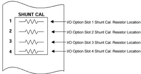
4. *FlexTest II*m/CTC Controllers only: Install the shunt calibration resistor into the **R-Cal** jacks in the appropriate DC conditioner.
