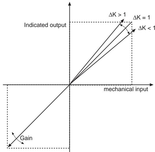
To calibrate the negative extensometer output:
