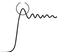
Here is a signal with a high degree of proportional gain. Derivative gain has not been applied yet. Notice how noisy the signal is.
