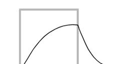
This waveform shows a sluggish (low gain) feedback signal.
