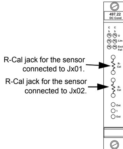
You also need to know which of the two DC conditioners on the module is used by your load cell.
