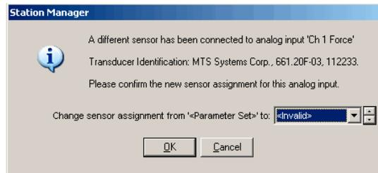
The sensor file list in this window only lists sensor files that match the basic TEDS information, conditioner type, and dimension. The sensor assignment window contains the same sensor assignment list found in the Station Setup window.
