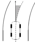
Note that error increases the longer the driver waits to correct it, that is, the larger the difference between the desired path and the actual path. The driver turns the steering wheel to adjust the car's path. But there is a problem.
