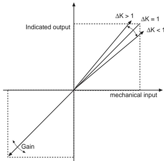
You should calibrate actuator extension at 80% of the full scale range.
