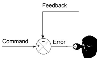
Derivative gain looks at the feedback side of the summing junction. It is the derivative of that signal, indicating how fast the feedback is changing.
