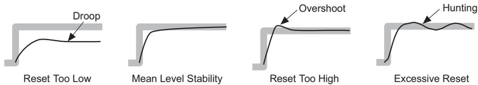
A ramp and hold waveform illustrate different levels of reset. The I Gain adjustment determines how much time it takes to improve the mean level accuracy.
