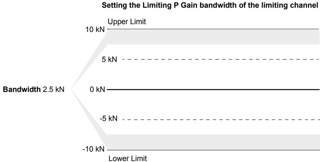
**Limiting P Gain** is turned on only within the upper and lower bands. The bands are defined by the **Bandwidth** control, as shown in the illustration.
