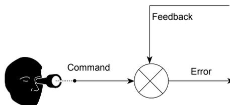
Feed forward gain looks at the command side of the summing junction. The output is the derivative of that signal, indicating how fast the command is changing.
